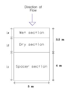
**Fig. 2.** Wet, dry, and spacer sections of a single cell with lengths *Lw*, *Ls*, and *Ld* with the solar panel covering the dry section
