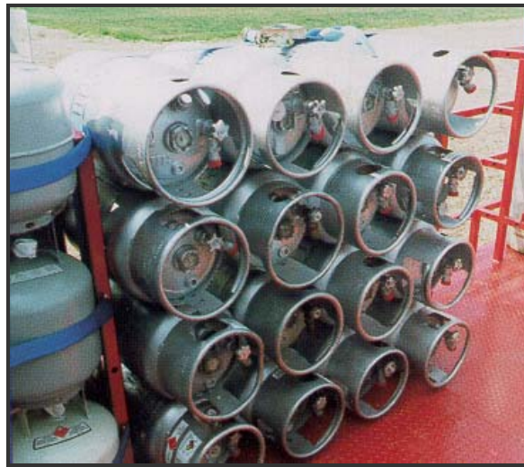
Figure 5.1.6c – Horizontally Secured Cylinders (Relief Valve at Top)
