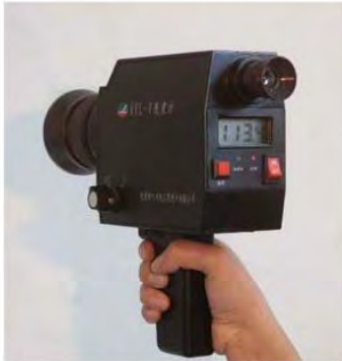
Figure 1 – A Typical Photometer (Shown reading 113.4 \text{cd}/\text{m}^2 )
