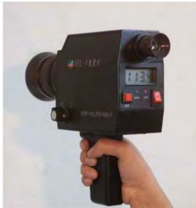
Figure 1 – A Typical Photometer (Shown reading 113.4 \text{cd}/\text{m}^2 )
