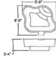
REGAL SPILLWAY - RGSW 600 Gal. Approx.
