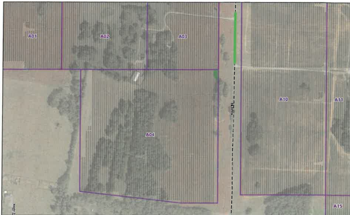
Figure 7: Route 03 with segments receiving glare (green lines) from Sub-Array A04
