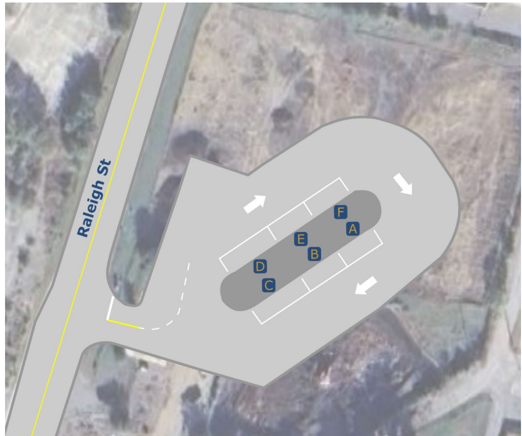
Figure 104 | Multimodal Transit Center Bus Loop Layout
