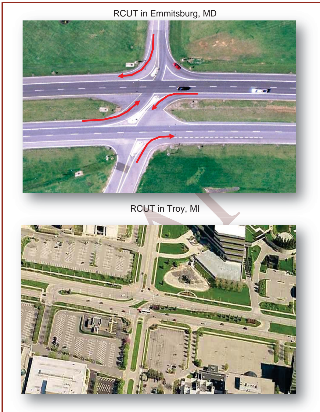
Figure 15: Examples of Restricted Crossing U-Turn (RCUT) Intersections, Source: Google Earth
